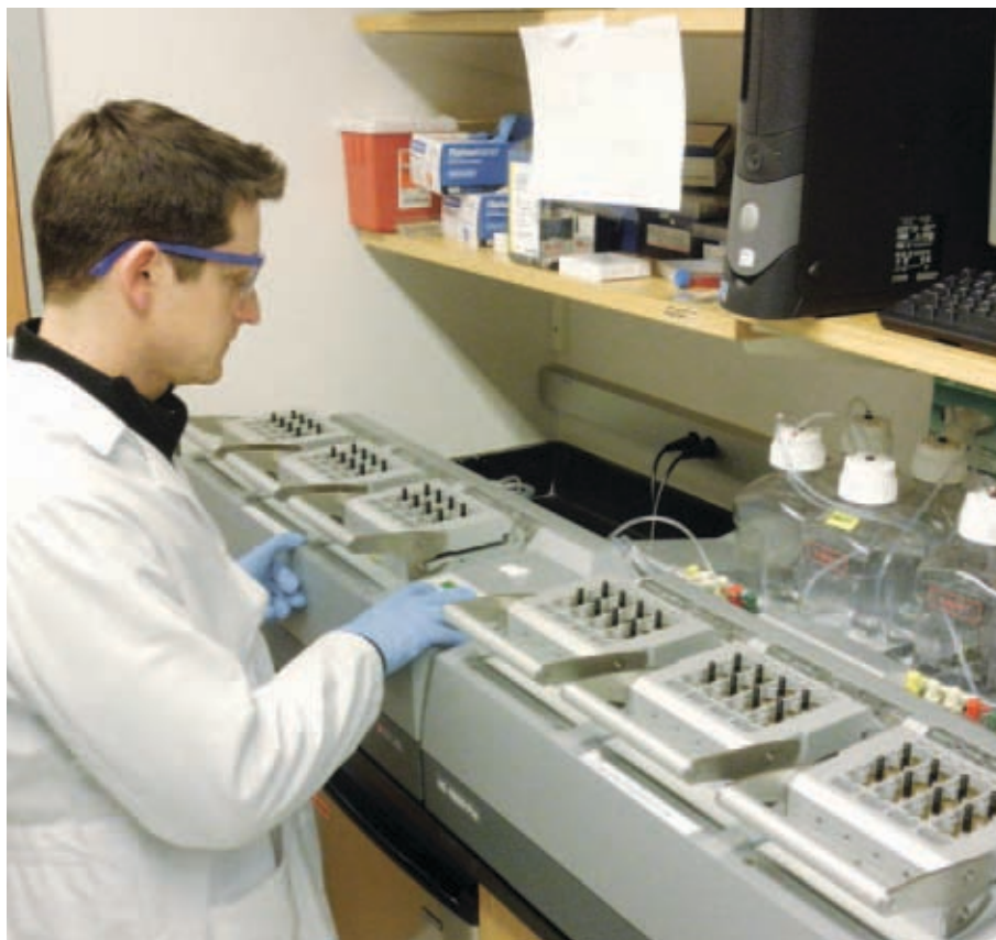
The HS 4800 Pro allows the Center for Neurologic Diseases to process up to 48 slides per run
