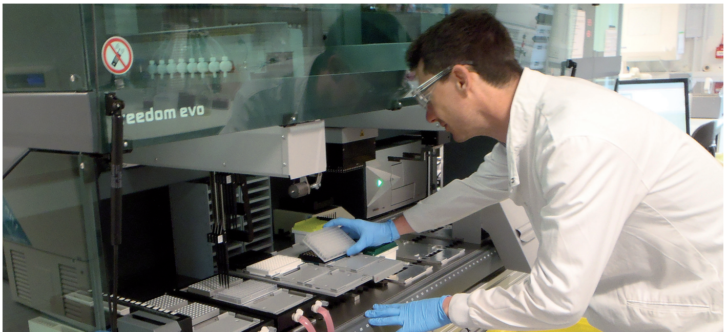
Isogenica's selection platform offers multiplexing capabilities in a 96-well format
