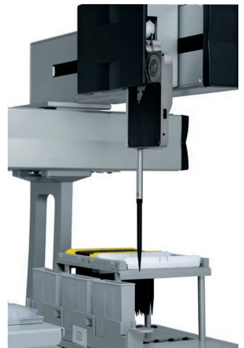
The Cavro Omni Robot ADP option offers maintenance-free pipetting
