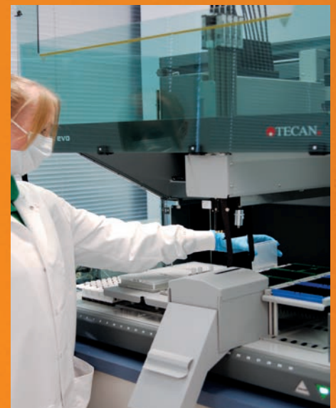
The Air LiHa offers precision liquid handling down to 1 µl
