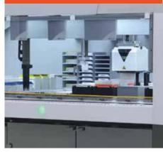
Simultaneous parallel movements of task-specific arms enhance speed and throughput
