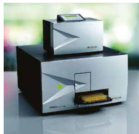
The GCM enables incubation of cell-based assays within the Infinite 200 PRO's measurement chamber
