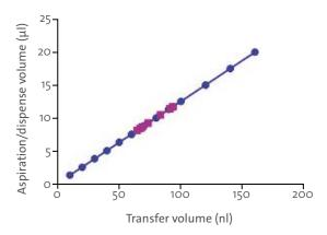
A calibration curve is performed for each assay buffer, demonstrating the excellent reproducibility of the liquid transfer technique
