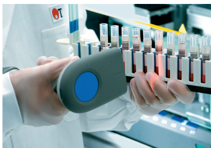
Hand-held barcode scanner for positive identification sample tubes
