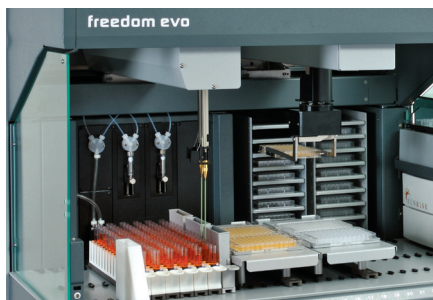
2-channel liquid handling arm with fixed washable tips
