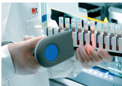
Hand-held barcode scanner for identification of samples and reagents
