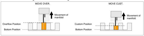
Figure 5.3 Movement Diagrams for Z-positions with MOVE
