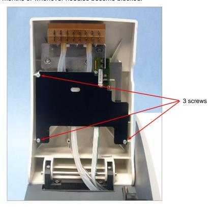
1. Lift the manifold arm and remove the black manifold arm guard plate by sliding it out from behind the three screws – the screws do not need to be removed to perform this step.
