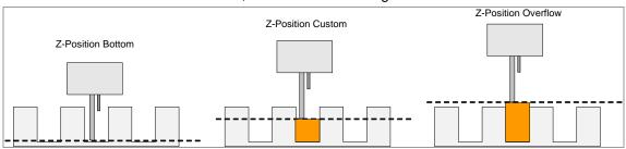
Figure 5.2 Z-Position Diagrams
