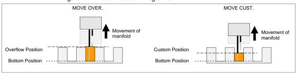
Figure 4.3 Movement Diagrams for Z-positions with MOVE
