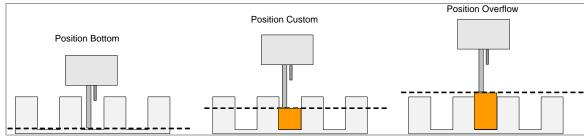
Figure 5.1 Aspiration Position Diagrams
