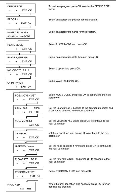
Figure 4.6 Example of a typical wash program for working with adherent cells
