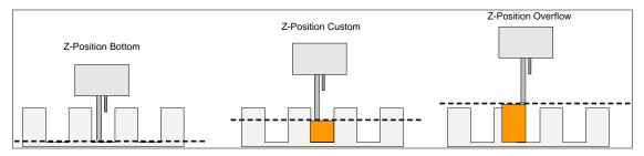
Figure 4.2 Wash Position Diagrams
