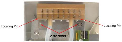
3. Tighten the manifold into place using the two screws using the Allen key provided.
