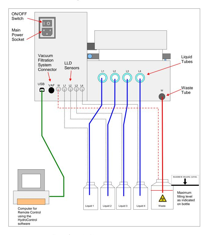
Fig. 3.2 Connection Diagram
