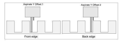
Fig. 4.5 Crosswise Aspiration for Flat Bottom Wells
