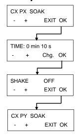
Select and confirm soak step (SOAK). CX = Cycle Number PX = Program Step Number
