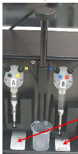
Figure 29: Injector-box with injector in 'service position'; the injectors are removed from the carrier slot and inserted into the holder of the injector carrier system.
