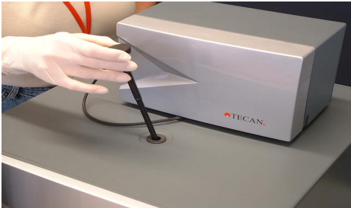
Figure 7: Inserting the injector carrier into the injector port
