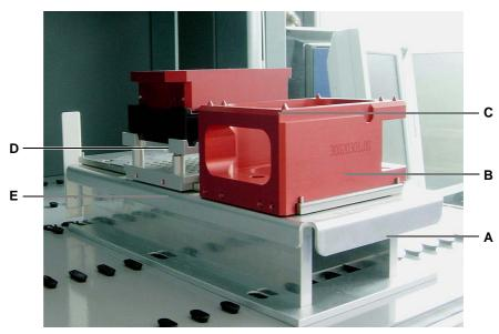
Fig. 8-186 Place tip / teach block on service carrier
