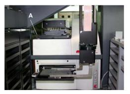
During this setup procedure the RoMa reference plate must be aligned with the tray (A) of the plate washer.
