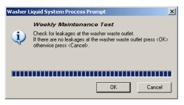
Fig. 10-129 Check washer waste outlet
