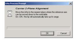
First, the Z-range is determined. The LiHa is automatically moved to an initial position. The prompt shown on the left along with the Move LiHa page appears.
