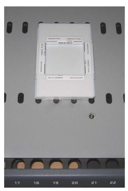
Place the reference plate on the worktable according to the grid position defined in the Setup page.
