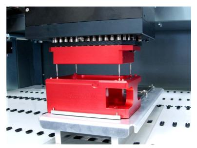
Fig. 8-190 Checking the alignment of the pipetting head
