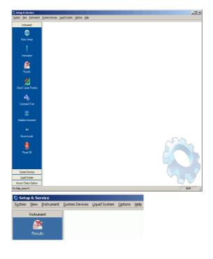
Setup and Service software communicates with the instrument and is in the Normal Mode of operation. The panel bar on the left side shows the panels of the active devices.
