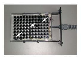
**Fig. 11-5** Temperature sensor plate (bottom view)
