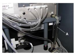
Fig. 10-128 Waste tubing reinstalled
