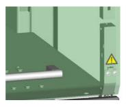
Door locks: During normal operation, they prevent the user from reaching into a zone in which movable parts like arm and pipetting devices are moving.
