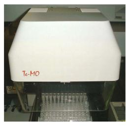
This pipetting head is equipped with 96 plungers and can aspirate and dispense liquid simultaneously through 96 channels. It is possible to attach a tip block with 96 tips or 96 DiTis to the head.
