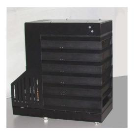
Heated incubator with shaker, calibrated to either 37 °C, 46 °C or 60 °C
