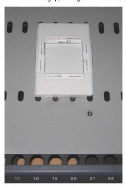
Place the reference plate onto the worktable according to the setting for Left Grid in the Test Configuration page.
