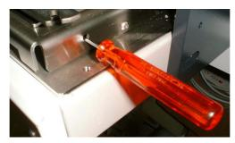
An APC rests on a ball-andsocket joint and can be turned in all axes. To level out an APC the fixing screw for the joint can be loosened and tightened when the adjustment is done.
