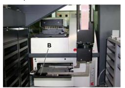
During this setup procedure the RoMa reference plate must be aligned with the tray (B) of the plate reader.
