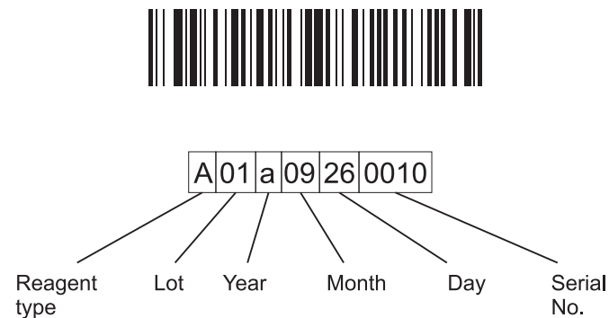
Fig. 12-6 Example of barcode masking
