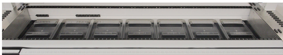
Fig. 20: Deck trays beneath the deck segments
