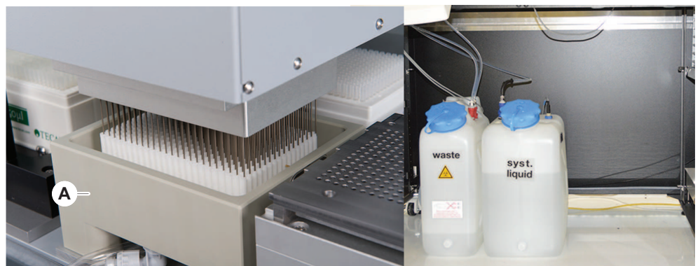
Fig. 29: Wash system (MCA)
