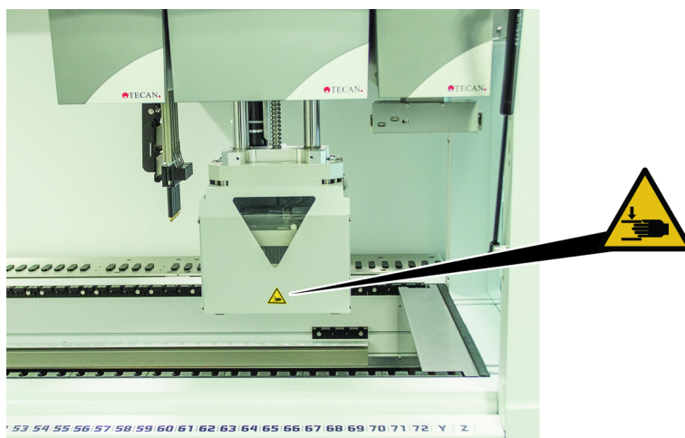
Fig. 11: Safety sign on MCA 384
