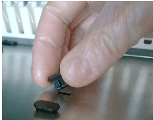
Fig. 7-34 Inserting a positioning pin
