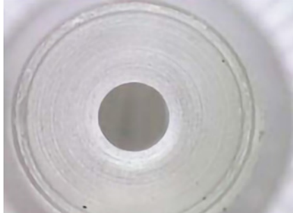
Figure 1. Magnified images of valve ports. Grooves visible as dark rings on the center and right images reveal damage due to overtightening.
