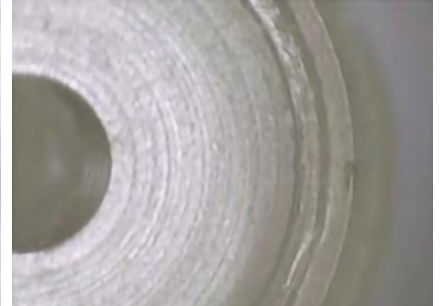
Figure 1. Magnified images of valve ports. Grooves visible as dark rings on the center and right images reveal damage due to overtightening.
