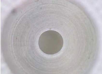
Figure 1. Magnified images of valve ports. Grooves visible as dark rings on the center and right images reveal damage due to overtightening.
