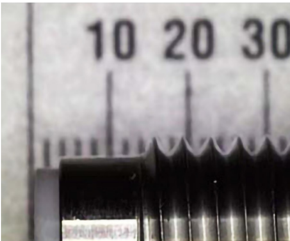
Figure 2. Magnified images of a new (left) and a worn (right) syringe. The thickness of the end cap is shown at the far left of the ruler.
