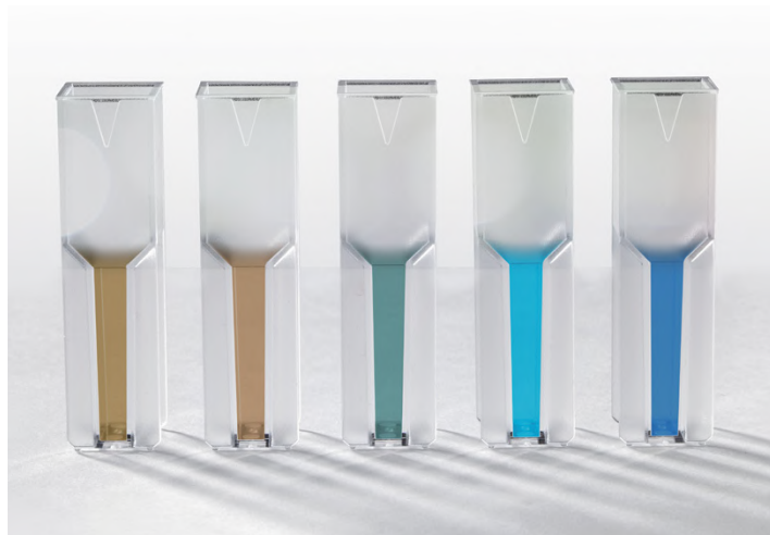
Figure 1: Bradford Protein Assay measured in cuvettes, showing increasing protein concentrations.
