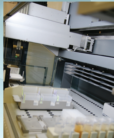
The Freedom EVO allows complete automation of the RoboColumns workflow
