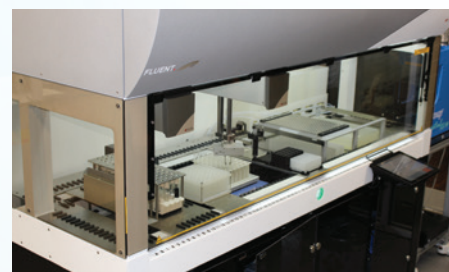
The Fluent Automation Workstation has been customized for GAP-PS peptide synthesis
