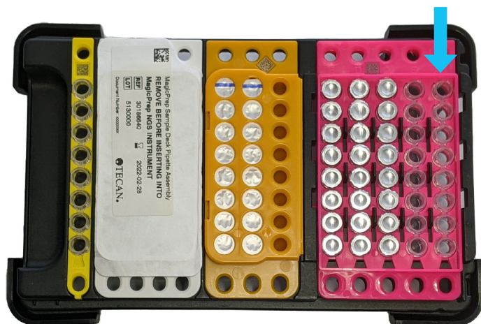
Figure 6. Top view of assembled sample deck. The tip assembly (white) is shown covered with the tip seal. When the sample deck handle is towards you, row A1 of the tube carrier assembly is on the left (blue arrow).
