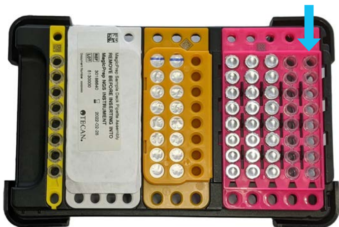
Figure 6. Top view of assembled sample deck. The tip assembly (white) is shown covered with the tip seal. With the sample deck handle facing towards you, row A1 of the tube carrier assembly is on the right (blue arrow).
