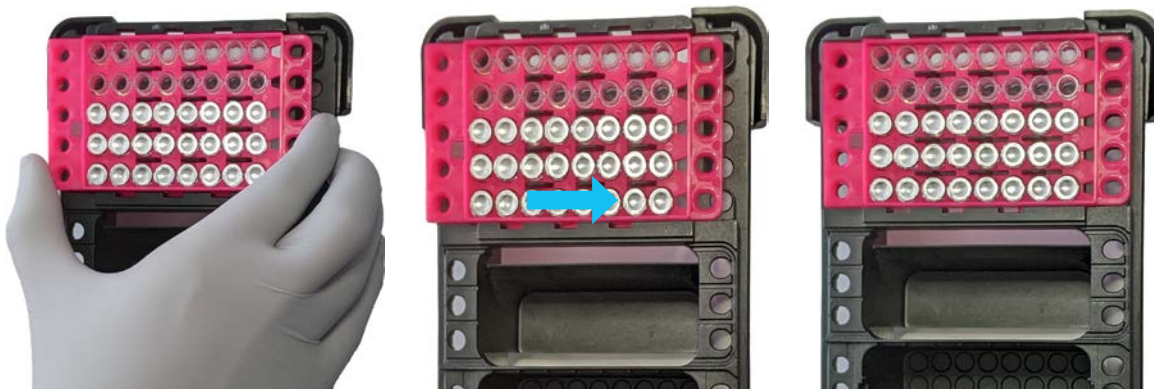
Figure 4. Inserting the tube carrier assembly. Align the tabs on the tube carrier assembly with the slots in the sample deck frame and push the tube carrier assembly down fully. Slide the tube carrier assembly so that rounded edges of the tube carrier assembly are flush with the side of the sample deck frame.
