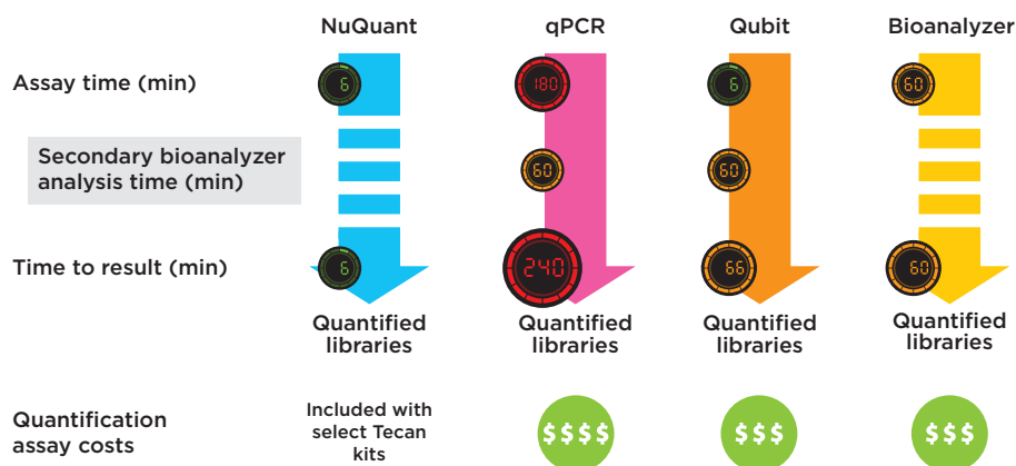
Figure 4: Library quantification workflow with NuQuant compared to qPCR, Qubit and Bioanalyzer. Following the recommended workflow for reliable library quantification by KAPA® Biosystems (Roche) [3, 4], qPCR library quantification can take up to four hours, whilst Qubit and Bioanalyzer analysis can take over an hour for results. NuQuant takes approximately six minutes for library quantification using a simple fluorometric assay, without the need for a separate fragment size analysis. Library quantification with NuQuant is included with certain Tecan kits, eliminating the additional cost associated with library quantification.
