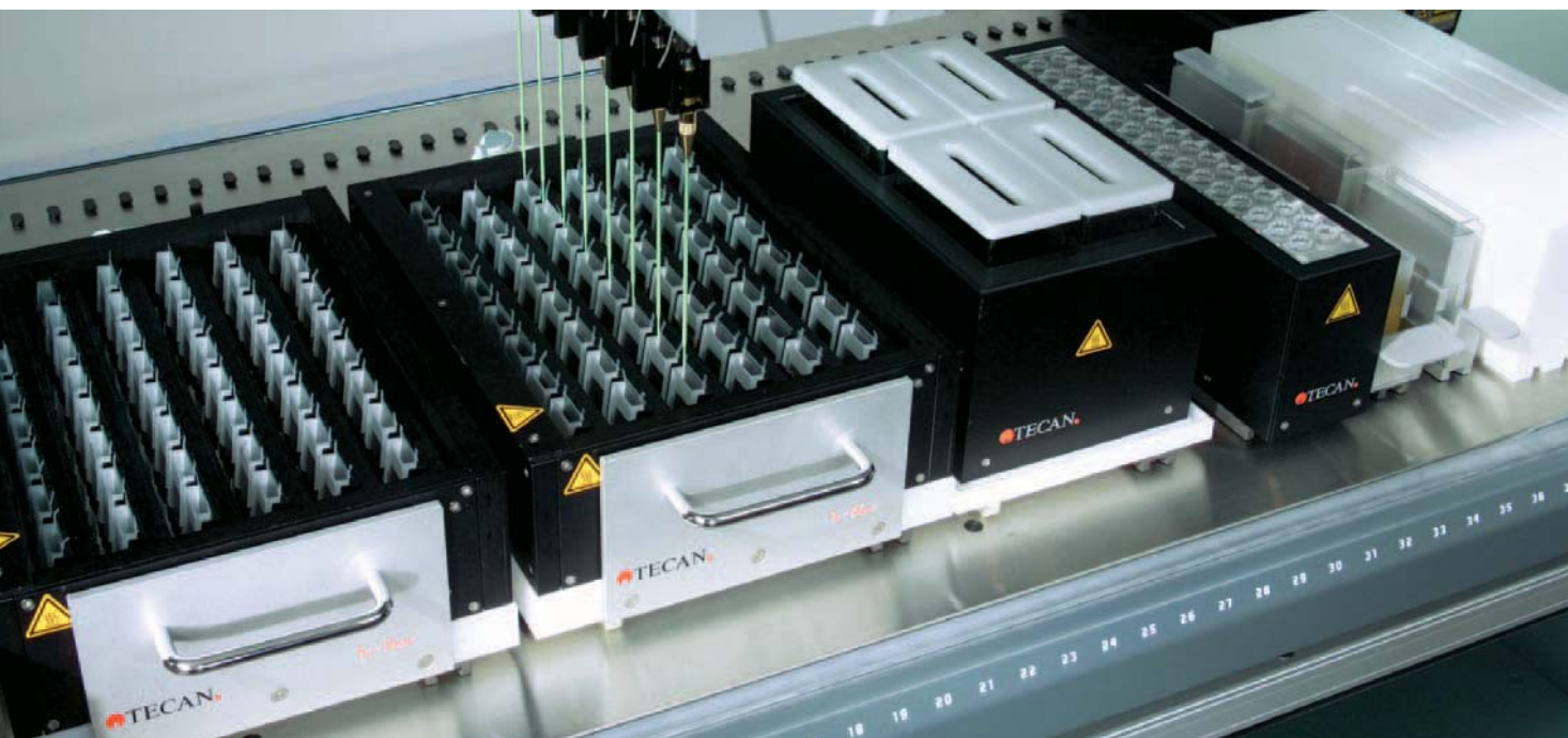
Figure 1: The GenePaint™ thermo-rack module for up to 48 hybridization chambers.
