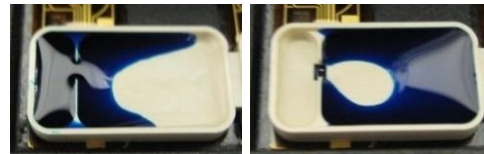
Good load Bad load Examples of good (left) and bad (right) load on high-volume cassettes.
