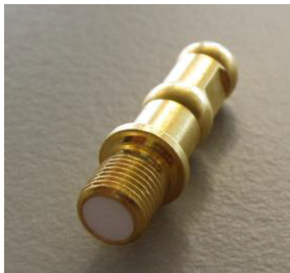
Fig. 127: DiTi cone with inline filter
