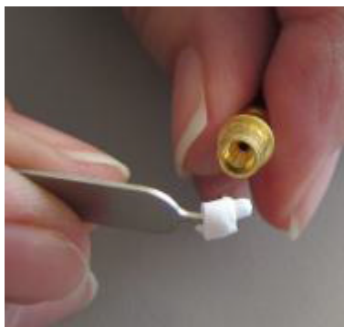
Fig. 125: Remove inline filter (2)
