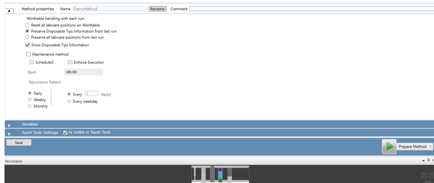
Fig. 94: Maintenance method: Lower pane of the Method editor
