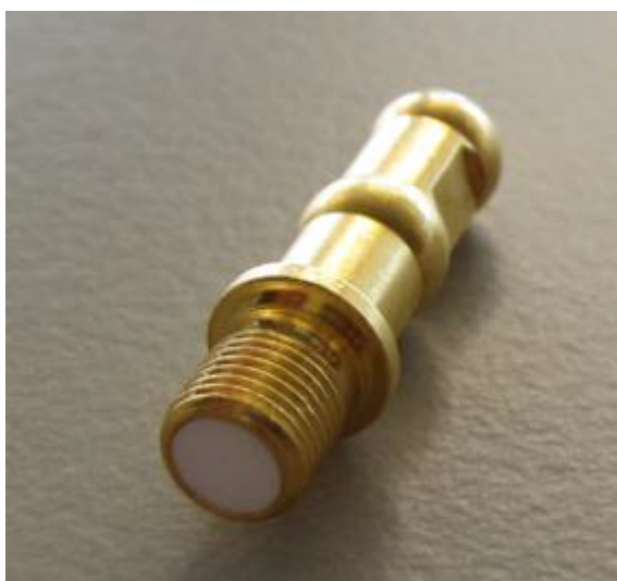
Fig. 134: DiTi cone with inline filter
