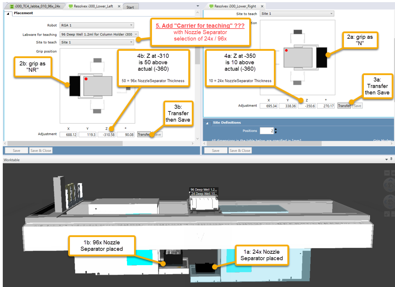
Fig. 249: Placement Resolvex i300 Nozzle Separator
