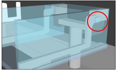
However, when pipetting with an MCA on a segment next to the FES segment you might get a collision error during runtime:
