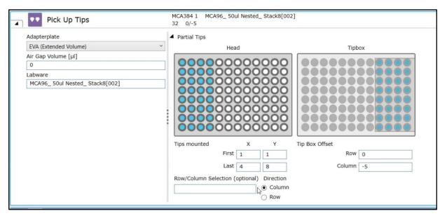
After an upgrade to FluentControl 3.4, any MCA384 "*Get Tips*" and MCA384 "*Drop Tips*" in existing scripts, processes or methods will be automatically renamed to MCA384 "*Pick Up Tips*" and MCA384 "*Set Tips Back*" respectively. No manual changes to scripts, processes or methods are needed.
