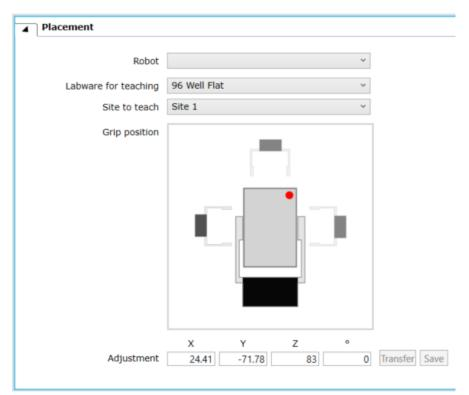
Fig. 1. Non-grid-based devices are taught using the Placement section of the device carrier definiltion. These values are stored on the instrument.
