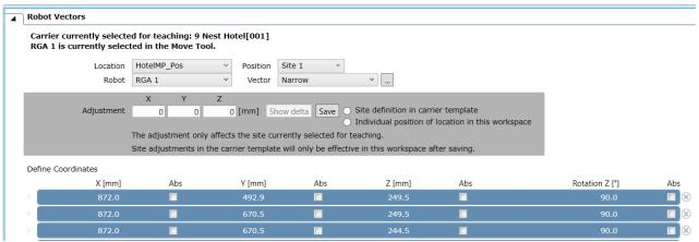
Fig. 2. Site-specific adjustments to carriers are stored on the instrument when the radio button 'Individual position of location in this workspace' is chosen.
