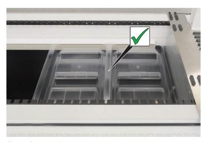
Fig. 43: Correct deck tray placement
