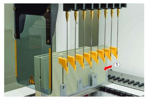
6. Unscrew the lock nut, holding the piercing tip immediately below the lock nut with the other hand.
