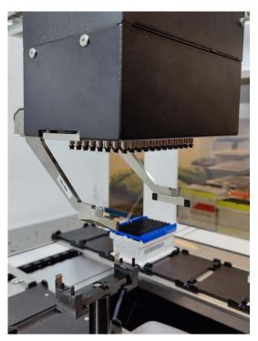
Fig. 23: MCA 96 Head / Gripper
