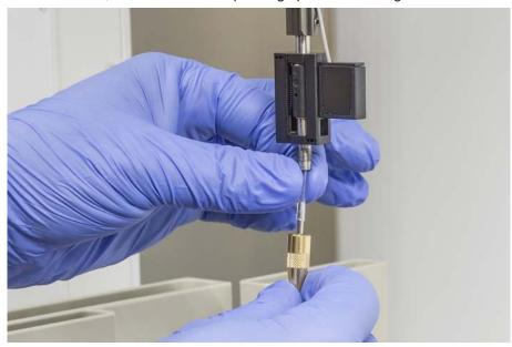
8. Insert the piercing tip and the pipetting tubing in the tip adapter.
