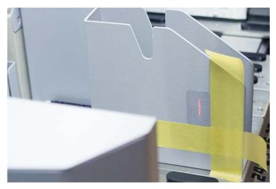
3. Remove the tape from the DiTi waste slide.
