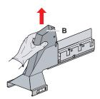
Fig. 48: Removing the disposable tip waste slide
