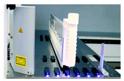
Fig. 38: Fluent ID LEDs
