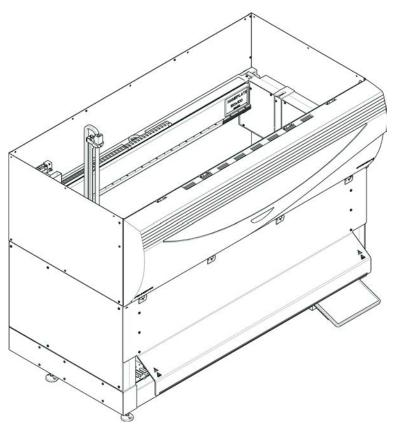
Fig. 4: Front Safety Panel with Expansion
