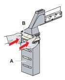
Fig. 53: Bag housing and disposable tip waste bag
