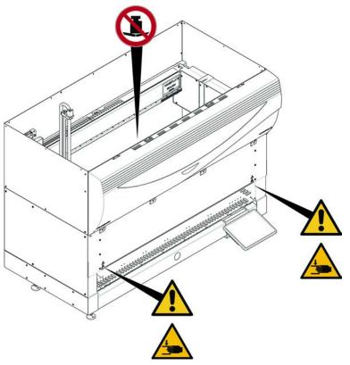
Fig. 9: Instrument with Half Front Safety Panel
