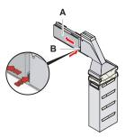
Fig. 44: Fastener for bag housing removal
