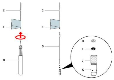
Fig. 62: Te-PS tubing widener
