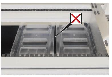
Fig. 41: Incorrect deck tray placement
