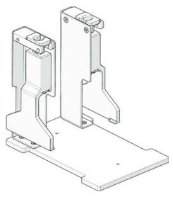
Fig. 28: FCA gripper
