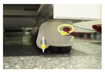
2. Loosen the locknut (A) on the corresponding foot.
