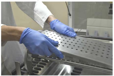
3. Clean the downholder plate according to the general instructions above or alternatively the tube downholder can be incubated in a bath with 2% bleach for maximal 2 hours.
