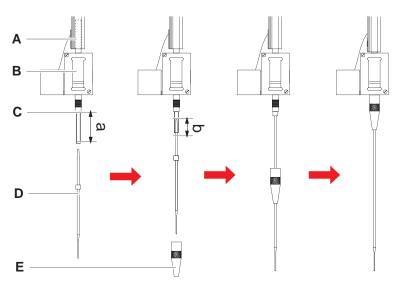
Fig. 61: Standard tip installation
