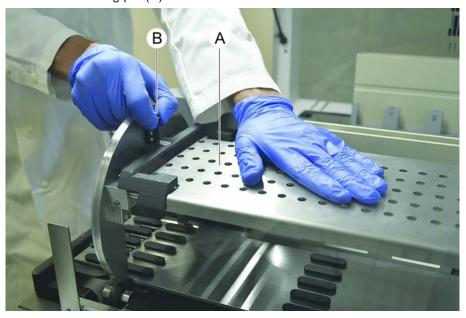
2. Remove the downholder plate from the tube rotator.
