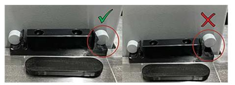
Fig. 54: Correct mounting of the waste chute on the worktable
