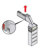
Fig. 45: Remove the wash station
