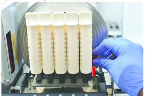
2. Pull the runner horizontally along the deck until it is fully removed.
