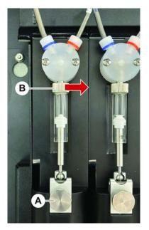
Fig. 56: Checking tightness
