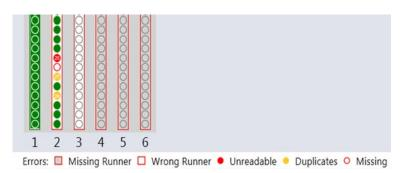
Fig. 40: Barcode reading confirmation displayed on the touchscreen
