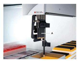
Fig. 22: Flexible Channel Arm
