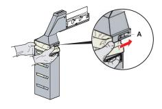
Fig. 52: Fastener for bag housing removal
