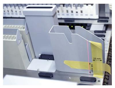
2. Apply the new self-adhesive reflector foil on the DiTi waste slide according to the illustration below.
