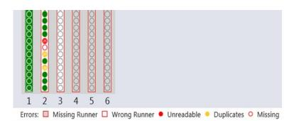
Fig. 39: Barcode reading confirmation displayed on the touchscreen
