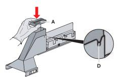
Fig. 51: Positioning pin and cover
