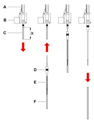
Fig. 64: Piercing tip installation
