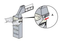
Fig. 55: Closing fastener
