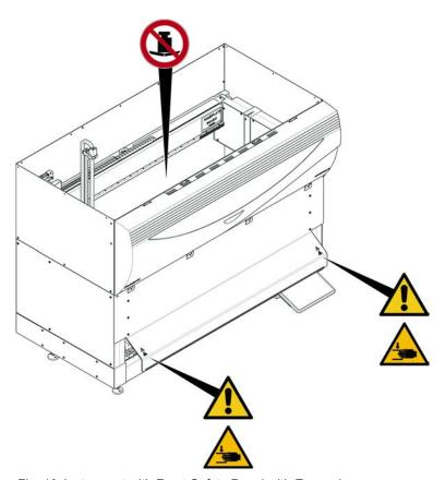
Fig. 10: Instrument with Front Safety Panel with Expansion
