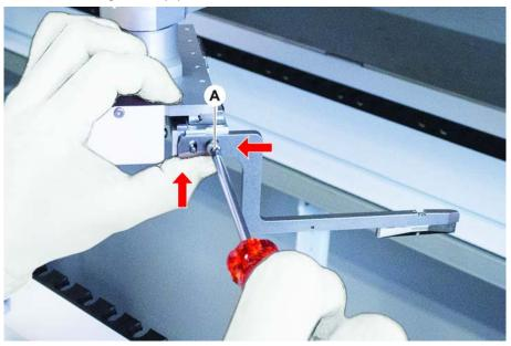
2. Press the Gripper Finger against the upper and the rear stop of the Gripper Head Mount and tighten the screw with a torque screw driver (3 or 3.5 Nm).
