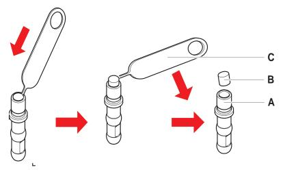
Fig. 59: Removing inline filter
