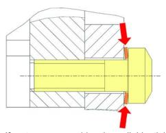
If no torque screwdriver is available, tighten screw until the washer is pressed flat and resistance increases. Then tighten  $^{1}/_{12}$  rotation further. This corresponds to approx. 3.5 Nm.
