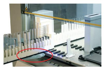
5. Slide the tube runners, one after another, onto the dedicated grids in the Fluent ID loading area.
