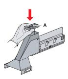
Fig. 47: Removing the cover from disposable tip waste slide
