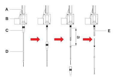
Fig. 60: Standard tip removal
