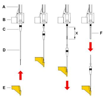
Fig. 63: Piercing tip removal
