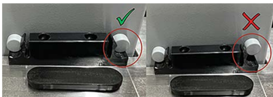
Fig. 57: Correct mounting of the waste chute on the worktable
