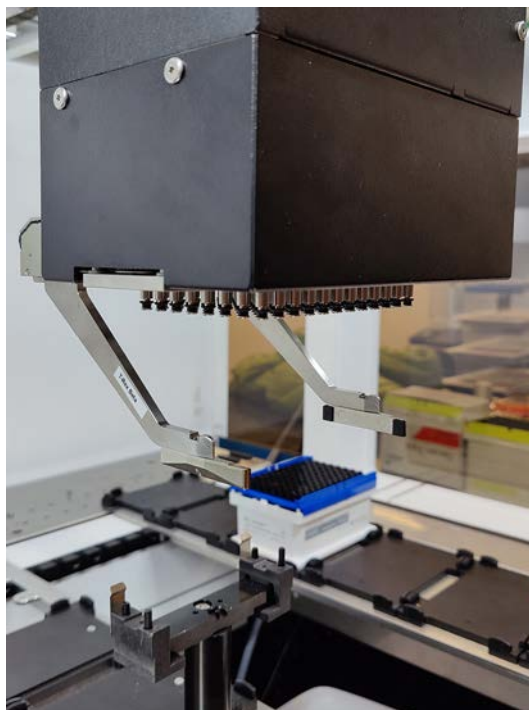
Fig. 25: MCA 96 Head / Gripper
