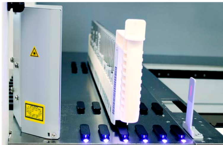
Fig. 41: Fluent ID LEDs
