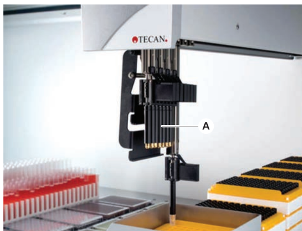
Fig. 23: Flexible Channel Arm
