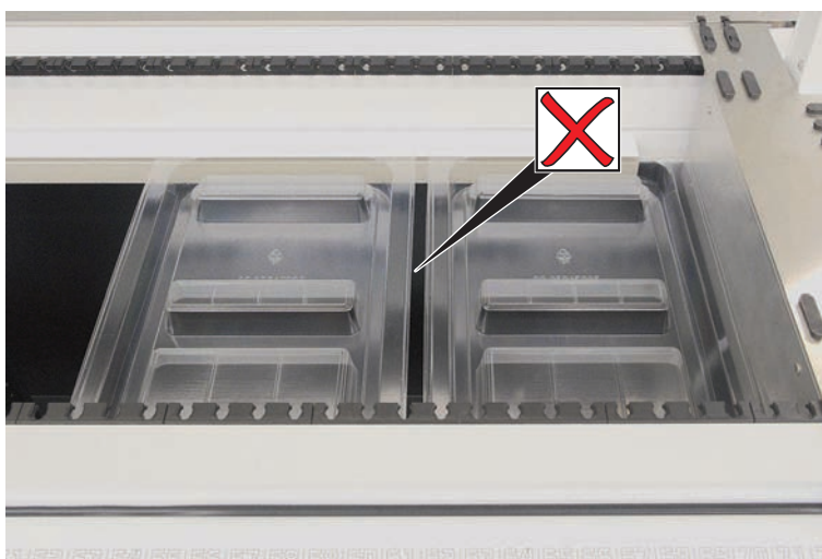
Fig. 44: Incorrect deck tray placement
