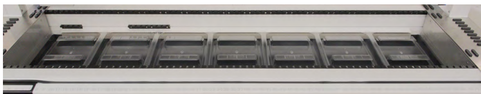
Fig. 20: Deck trays beneath the deck segments
