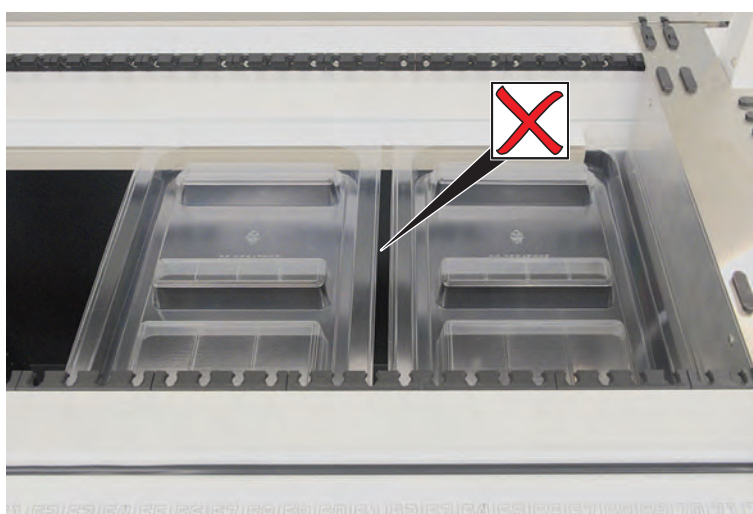
Fig. 42: Incorrect deck tray placement
