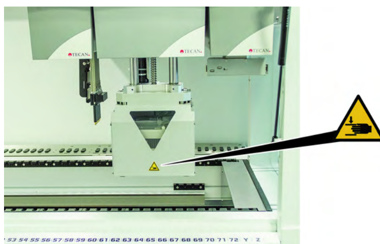
Fig. 11: Safety sign on MCA
