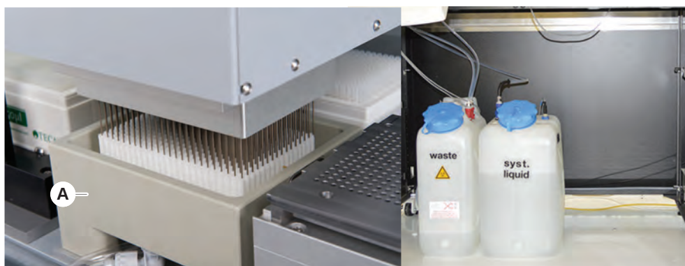
Fig. 28: Wash system (MCA)
