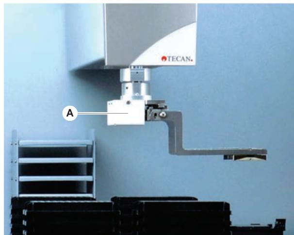
Fig. 26: Robotic Gripper Arm
