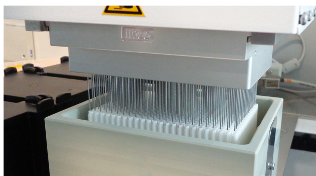
Fig. 3-13 Adapter Fixed 15 µl MCA384
