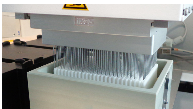
Fig. 3-14 Adapter Fixed 125 µl MCA384
