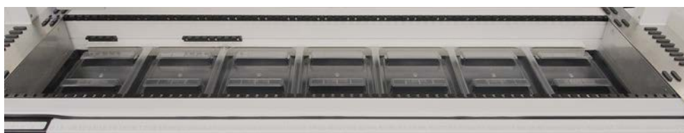
Fig. 19: Deck trays beneath the deck segments
