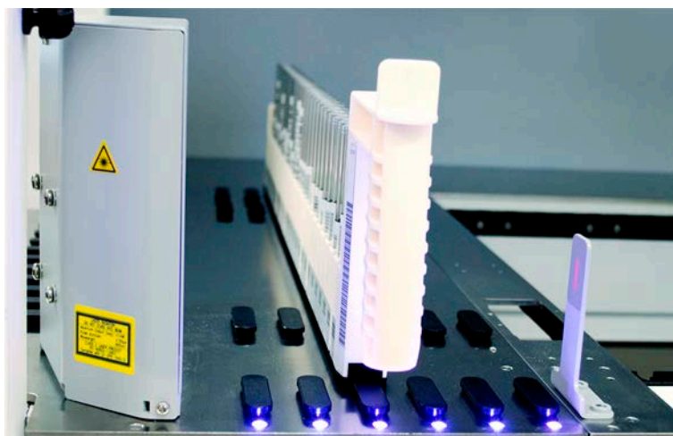
Fig. 38: Fluent ID LEDs
