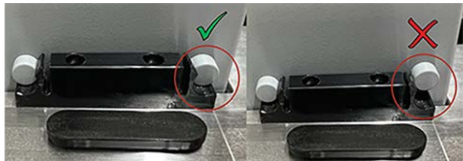
Fig. 54: Correct mounting of the waste chute on the worktable
