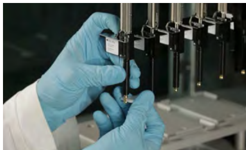
Fig. 7-10 DiTi cone wrench
