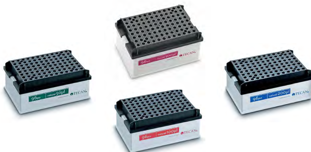
Fig. 4-48 DiTi boxes with 50 µl, 100 µl, 200 µl and 500 µl DiTis
