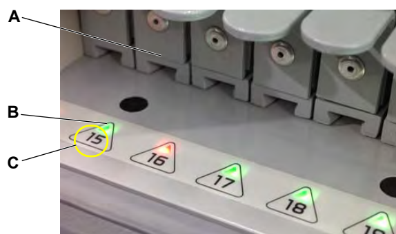
Fig. 6-3 Indicator LEDs of the loading interface
