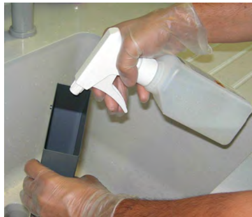
Fig. 7-22 DiTi waste slide
