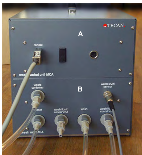
Fig. 4-32 Wash System MCA
