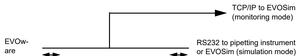
Fig. A-44 Principle of the data splitter tool EVOSim Splitter
