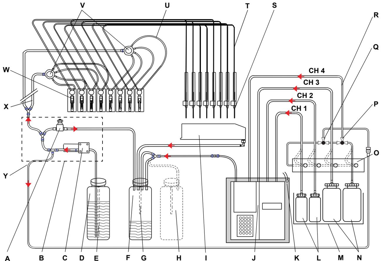
**Fig. 4-2** Overview of typical 8-tip configuration
