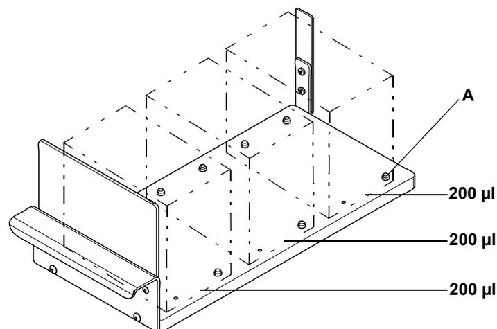
**Fig. 11-4** Carrier for DiTi racks (3 DiTi racks 200 µl)
