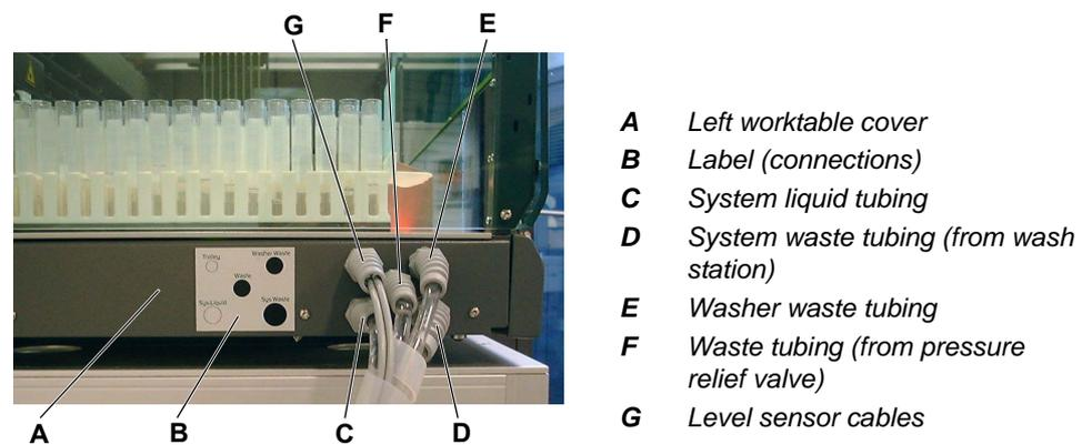
**Fig. 7-3** Tubing/cables to containers
