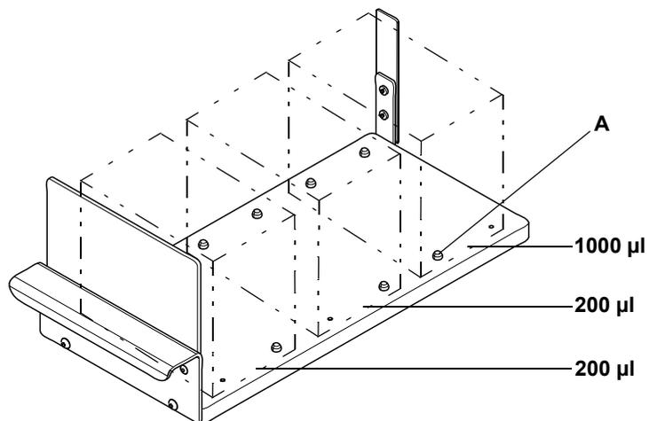
**Fig. 11-5** Carrier for DiTi racks (2 DiTi racks 200 µl, 1 DiTi rack 1000 µl)
