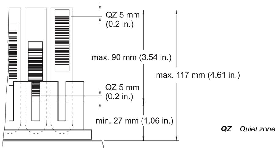
**Fig. 3-7** Barcode label on tubes
