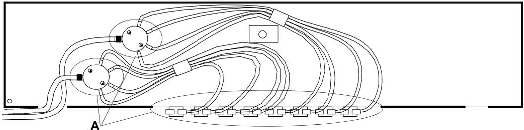
**Fig. 7-1** Tubing connections (top view of instrument)
