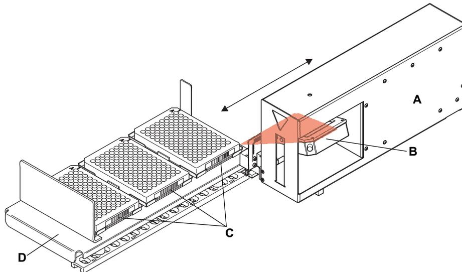
**Fig. 4-13** Barcode scanner position for scanning horizontal barcodes
