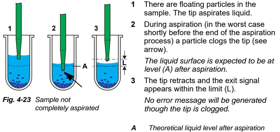
**Fig. 4-23** Sample not completely aspirated
