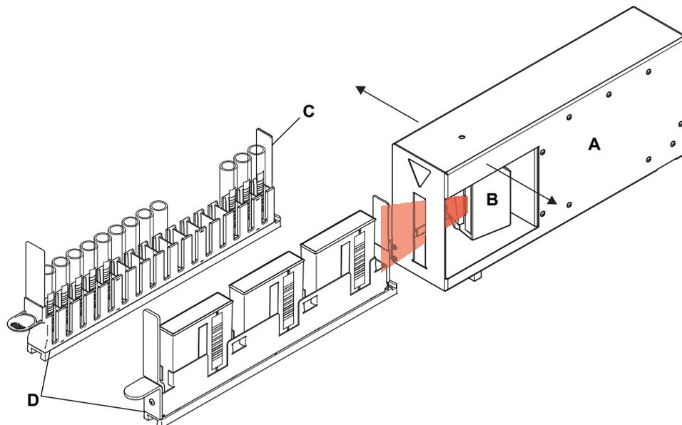
**Fig. 4-11** Barcode scanner position for scanning carrier ID
