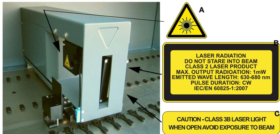
Fig. 2-2 Laser labelling on PosID
