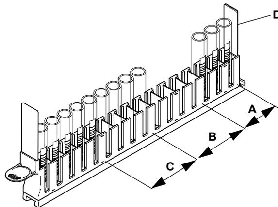
**Fig. 4-14** Detectable situations in a tube rack
