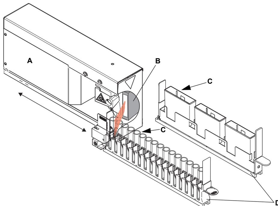
**Fig. 4-12** Barcode scanner position for scanning vertical barcodes
