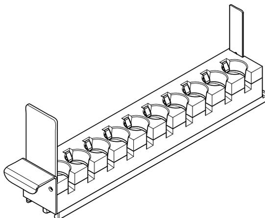
**Fig. 11-11** Carrier with 10 pos. for reagents / controls
