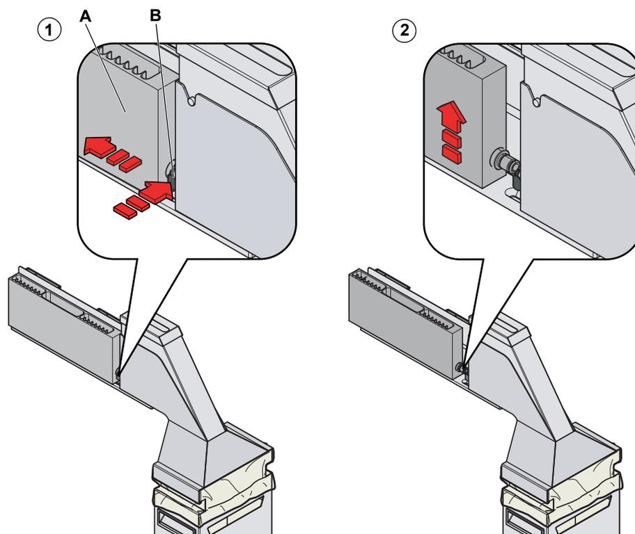
Fig. 7-21 Removing the wash station from the worktable
