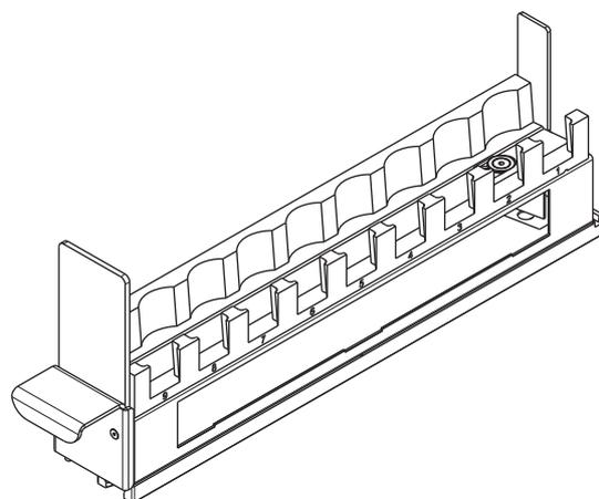
**Fig. 11-14** Carrier for reagents 9 pos.
