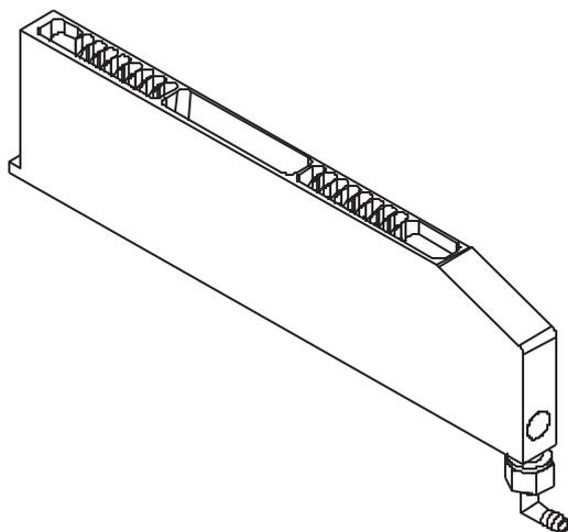
**Fig. 11-18** Wash/waste station, standard
