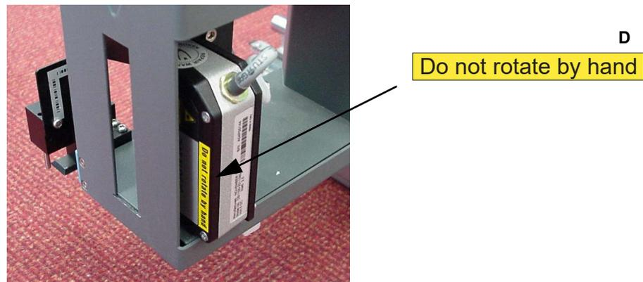
Fig. 2-3 Label on PosID scanner head
