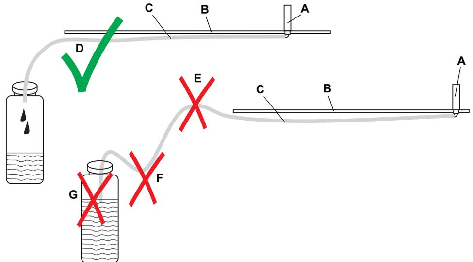
**Fig. 7-13** Correct and disadvantageous course of waste tubing
