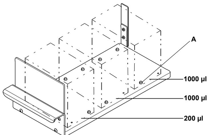
**Fig. 11-6** Carrier for DiTi racks (1 DiTi rack 200 µl, 2 DiTi racks 1000 µl)
