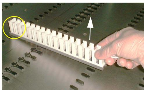
**Fig. 7-33** Extracting a positioning pin
