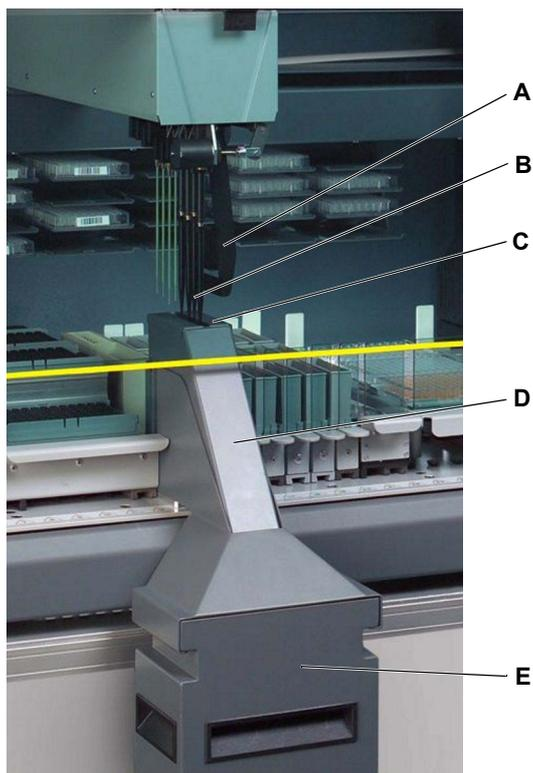
**Fig. 4-26** Lower DiTi eject option with cover and waste slide
