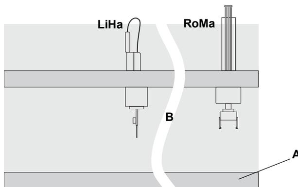
**Fig. 3-6** Arm configurations of the Freedom EVOlyzer
