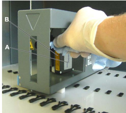
**Fig. 7-27** PosID barcode scanner
