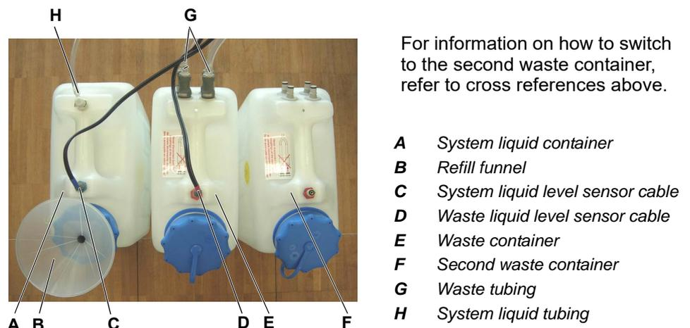
**Fig. 7-4** Container connections
