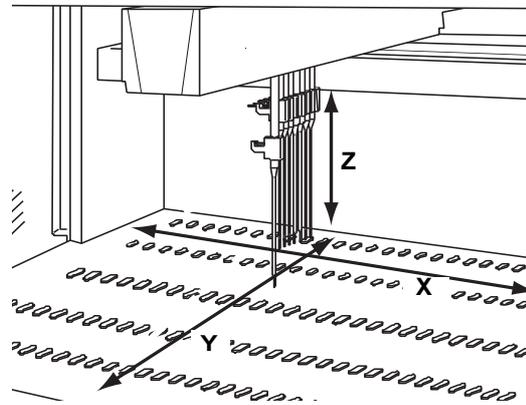
**Fig. 4-4** Liquid handling arm movement
