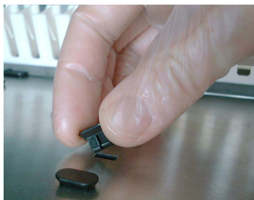
Fig. 7-34 Inserting a positioning pin
