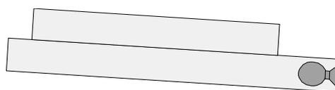
4. Carefully slide the plate carrier with the prime tray at the rear over the guide bar.
