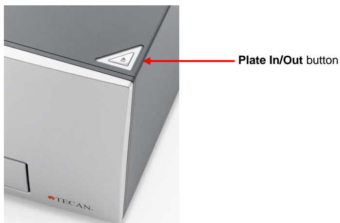
Figure 1: Onboard of the Infinite reader. The Plate In/Out button is in the front right corner of the top cover.
