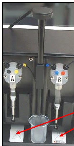
Figure 29: Injector-box with injector in service position ; the injectors are removed from the carrier slot and inserted into the holder of the injector carrier system.
