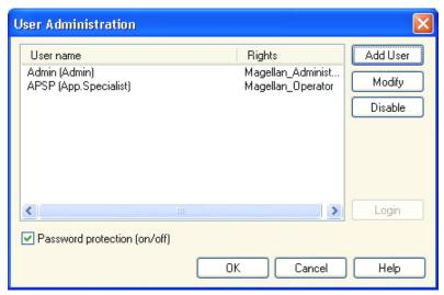
User profiles can be defined at three different security levels. The highest level of security within the software is that of the **magellan Administrator**. This level gives access to all the program's functions and data editing facilities. For **Application Specialist** and **Operator** level, options are increasingly restricted.
