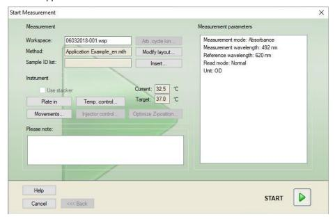
Click **Start** to start the measurement. A workspace will be created automatically, which contains all previously entered information and will collect all measurement values. While the measurement is being executed, a measurement status dialog box appears indicating the progress of the measurement.
