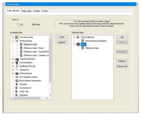
On the **Data selection** tab, all available report data is contained in the **Available data** box. Using the **Insert and Append** buttons, data can be transferred into the **Selected data** box. Data can also be transferred using drag-and-drop. In the **Print as** box, choose between printing the data as a matrix or as a list with a special orientation.
