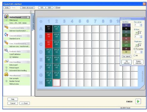
Click **Select all unused** from the toolbar to select all empty wells on the plate. Then hold down the control (Ctrl) key and click the well **H12**, so that it remains blank and unmarked.
