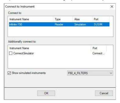
For demo mode select the **Show simulated instruments** checkbox and the preferred instrument from the drop-down list, click the instrument name and click **OK**.
