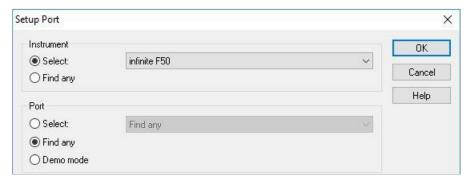
Select **INFINITE F50** in the **Instrument** group box in the **Setup Port** dialog box. Click **OK** to display the **Connect to Instrument** dialog box.
