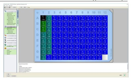
In each single well the calculated value is displayed. Depending on the selected item in the control bar, the plate layout window changes correspondingly. Parameters and settings can be changed using the items in the control bar. If the method is to be modified, click on the **Edit method** tab.
