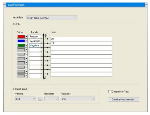
Click **Cutoff results selection** to select the identifier types for which the cutoff results must be shown.
