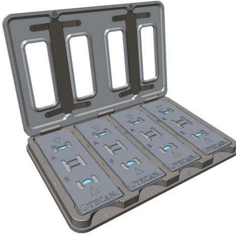
Figure 72: Cell chip adapter with springs (dark gray)
