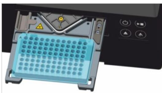
Figure 2: Microplate on the plate carrier with the A1 well in the upper left-hand corner
