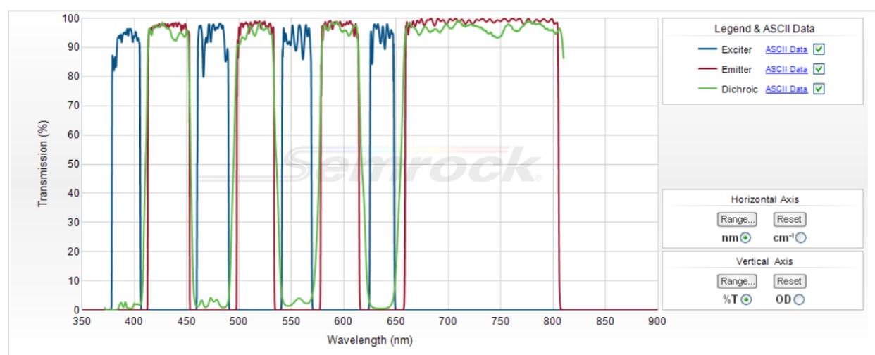
Figure 16: Transmission profile of the full-multiband filter set, built-in T-image (obtained from the official Semrock website: [www.semrock.com](http://www.semrock.com)).
