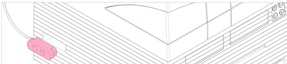
Figure 25: Condensation prevention stoppers (both sides of the instrument)
