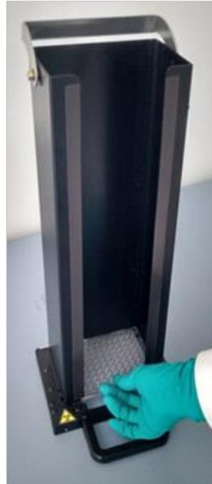
1. Manually insert the microplate into the top of the plate magazine and carefully lower it towards the bottom of the stack.
