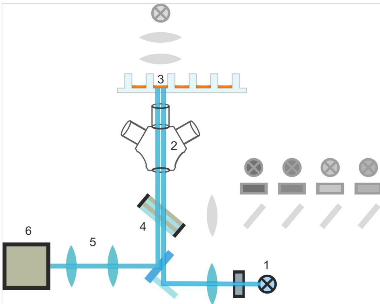
Figure 14: Schematic diagram of the auto-focusing system
