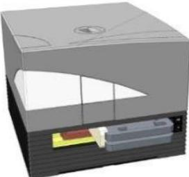
7. Insert the piece of foam into the left plate carrier compartment (see picture below).
