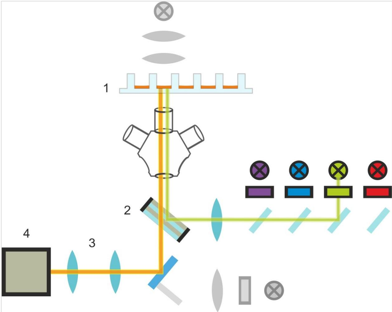
Figure 15: Schematic diagram of the fluorescence illumination system
