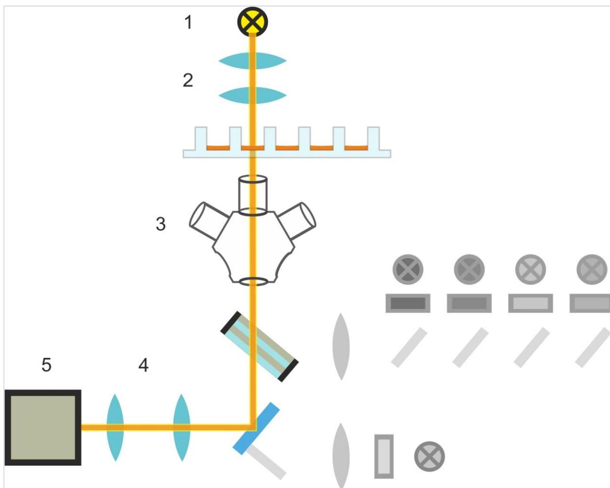
Figure 13: Schematic diagram of the bright field illumination system
