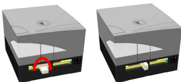
4. Move the plate carrier out carefully by hand until it lightly presses against the inserted white piece of foam from behind and cannot be moved out further.
