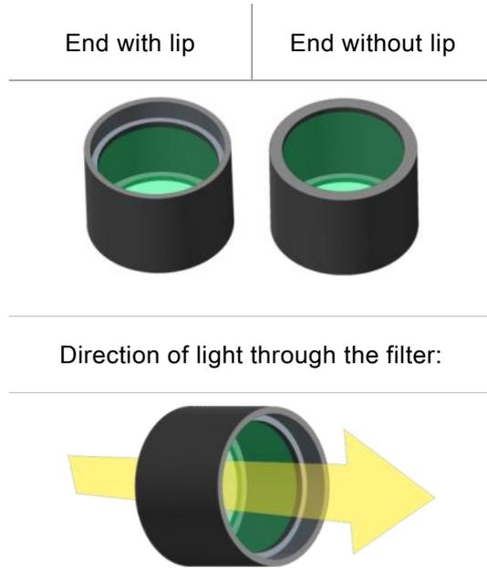
Figure 8: The light travels from the end without the lip towards the end with the lip.
