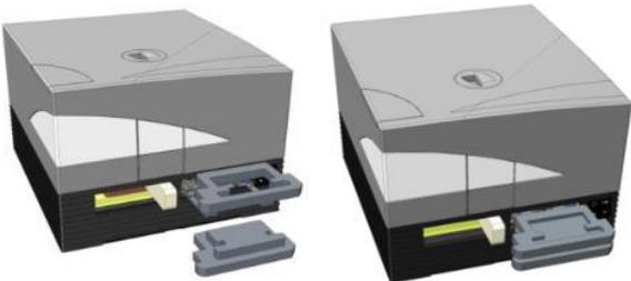
6. Move the plate carrier into the right compartment manually as far as it can go by pushing on the pieces of foam on the plate carrier.
