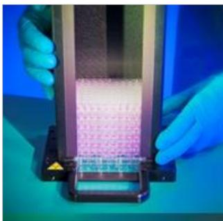
4. Lift up the plate magazine. The stack of microplates has been added to the plate magazine. The platform plate remains on the lab bench.
