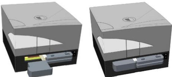
8. Tape the filter compartment doors shut (see picture below).
