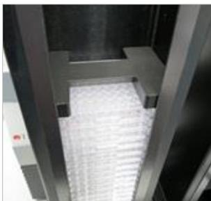
2. Place a stabilizer weight at the bottom of the output magazine.
