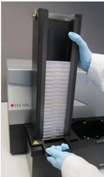
3. Load the empty plate magazine at the position labelled OUTPUT.
