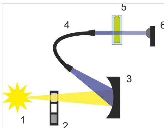
Figure 7: Optical system of the absorbance cuvette module
