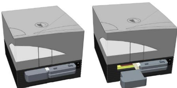
4. Move the plate carrier out manually by pulling on the pieces of foam in the right plate carrier compartment (see picture below).
