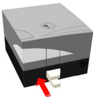
3. With the foam piece inserted, turn it 90° clockwise, so that the pointed end sticks down into the space between the two compartment openings. This piece of foam holds the compartment doors open.
