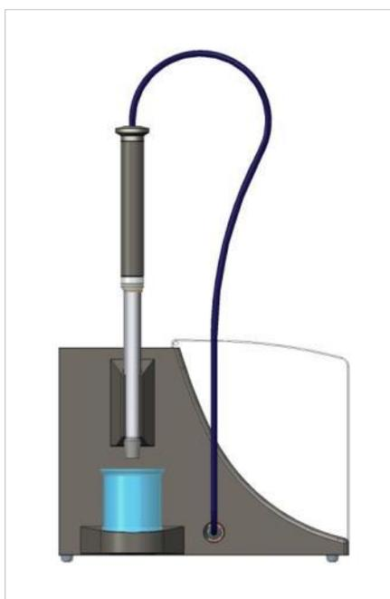
Figure 20: Injector carrier in service position
