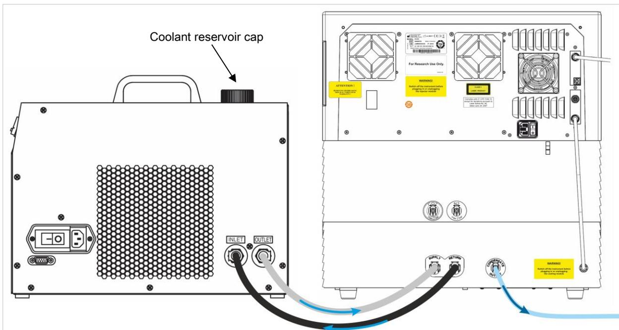
Figure 21: SPARK with integrated cooling module connected to the external liquid cooling device
