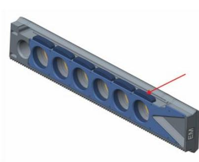
Figure 10: Remove the filter by pushing the button next to the appropriate filter slot (see picture above), turn the filter slide over and the filter will slide out of the slot.
