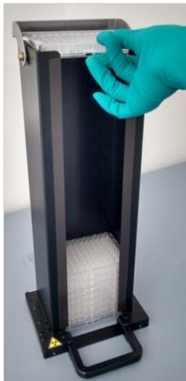
2. Carefully grip the microplate at the top of the stack of plates in the plate magazine.
