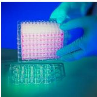
3. Slide the plate magazine over the stack of microplates all the way down until the plate magazine makes contact with the surface of the lab bench.
