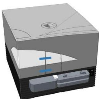
3. Remove the piece of foam from the left plate carrier compartment (see picture below).
