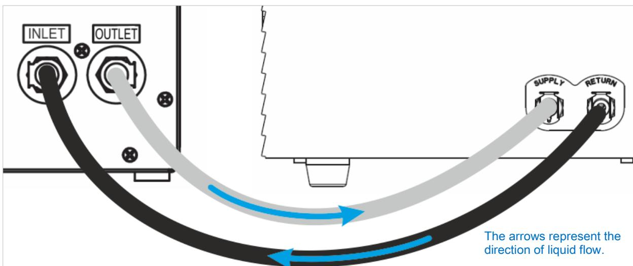
Figure 22: Connections between the integrated cooling module and the external liquid cooling device
