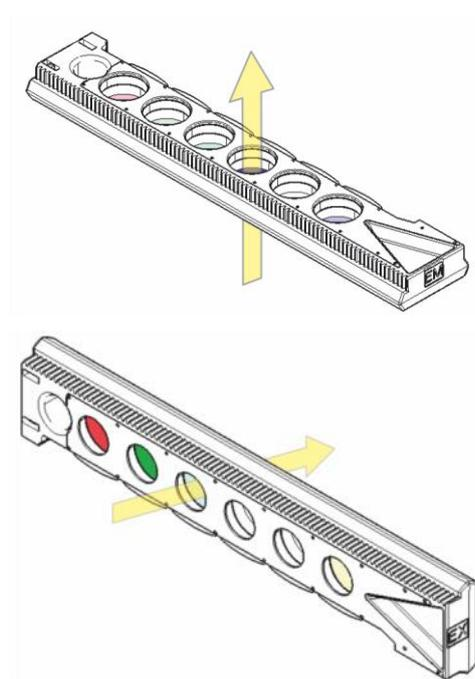
Figure 9: Direction of light through the filter slides
