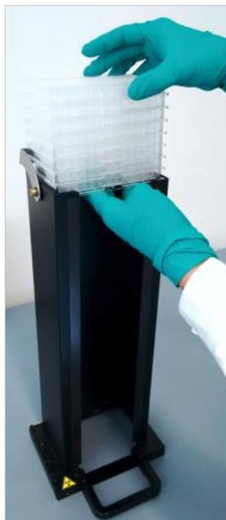
3. Carefully slide one hand underneath the microplate at the bottom of the plate magazine and stabilize the group of microplates you want to unload, with the other hand.
