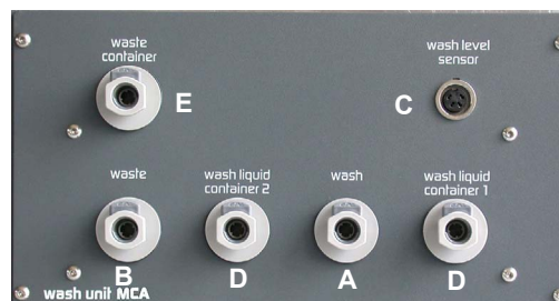
Fig. 5-11 Wash unit MCA
