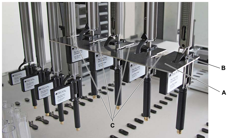
Fig. 7-9 Insertion of adjustment gauge for Air LiHa tip adapters
