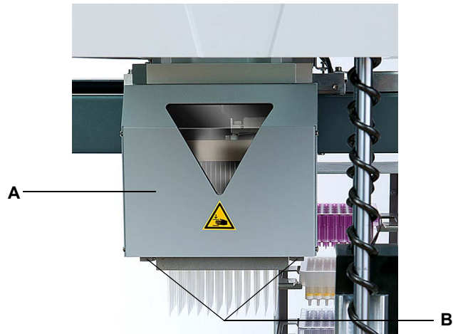
Fig. 2-5 Safety covers on 384 channel pipetting head
