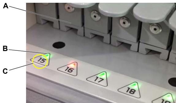
Fig. 6-3 Indicator LEDs of the loading interface
