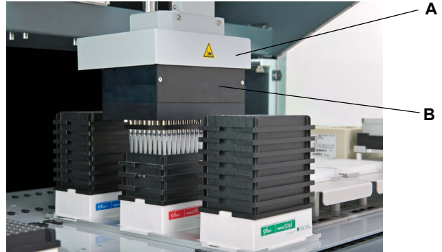
Fig. 2-4 Safety elements/covers on 96 channel pipetting head
