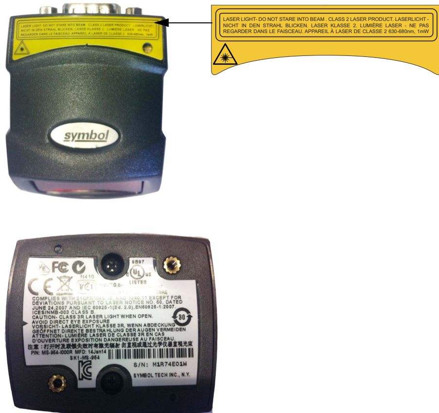
Fig. 2-14 Laser labelling on the symbol BC scanner
