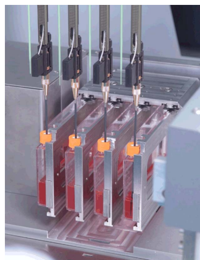
Fig. 4-92 Flask flipper in vertical position for septum piercing and pipetting
