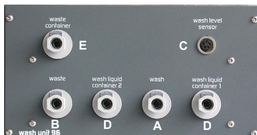
Fig. 5-8 Wash unit MCA
