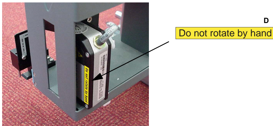
Fig. 2-12 Label on PosID scanner head
