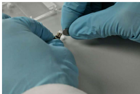
Fig. 7-14 Inline filter removal
