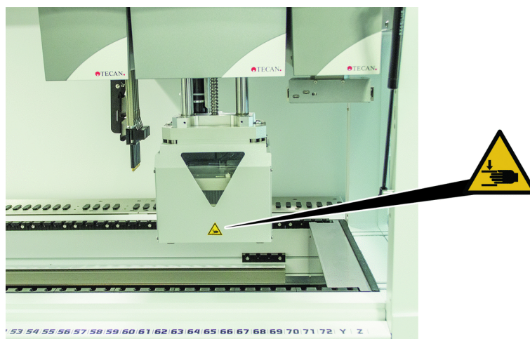
Fig. 11: Safety sign on MCA
