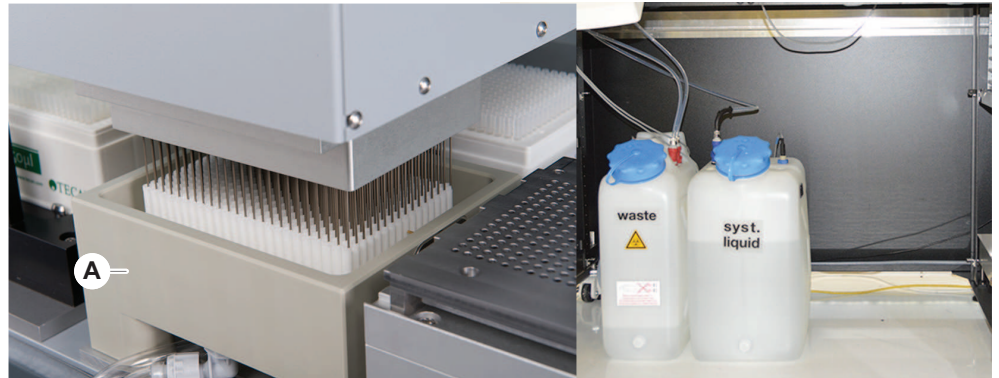
Fig. 28: Wash system (MCA)
