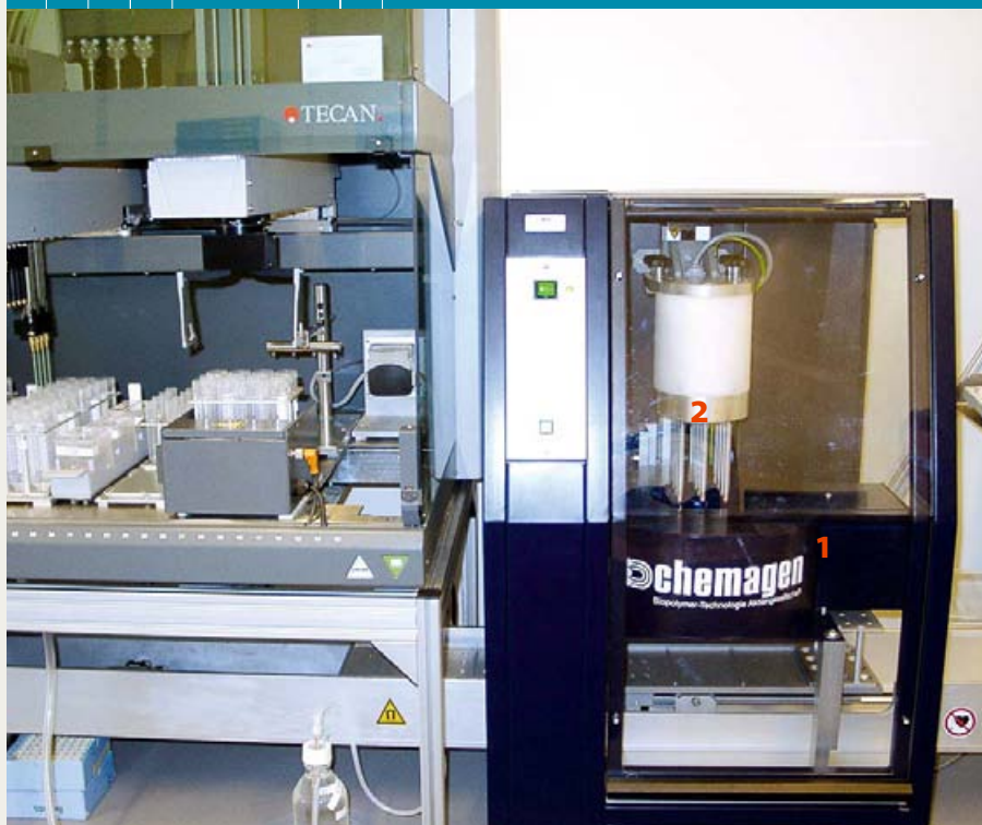
Figure 3: Chemagic Magnetic Separation Module I (Chemagen). Electromagnet [1] and metal 12-rod head [2].
