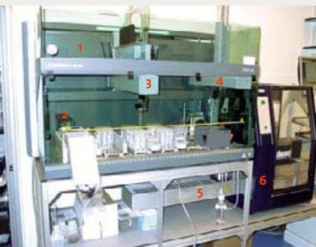
Figure 1: Fully automated DNA extraction set-up: Tecan Freedom EVO 150 Workstation and Chemagic Magnetic Separation Module I (Chemagen).
