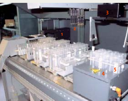
Figure 2: Fully automated DNA extraction set-up in detail.
